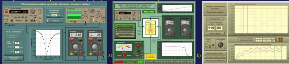
Fig. 3 Users interfaces of the experiments appointed to: a) electrical resonance b) Curie temperature determination for ferromagnetic materials c) heat conductivity studies with the Ångström method.
